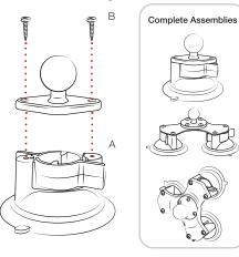
Clean surface thoroughly. Align the suction cup to surface. While holding the lever to the OFF position, push the plastic base onto the surface flush with the silicon base and switch the lever to the lock position. Suction cup base must be locked flush with the silicon for a successful hold.
