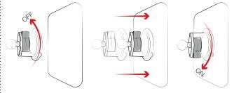
RAM® Twist-Lock™ Suction Cups are only compatible with smooth, non-porous surfaces (no rough or textured surfaces). Clean surface thoroughly before applying suction. When left unattended in extreme temperatures, it is recommended to remove and stow suction cups. Suction cups are considered a general wear item and are not covered under any warranty.
